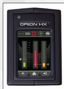
Tx and Rx graph displays power, 2nd, and 3rd harmonic levels and touch screen trip and power level adjustments.
