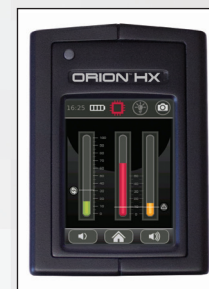
Histogram graph displays history of harmonic response and power adjustment from 10 - 60 second duration.
