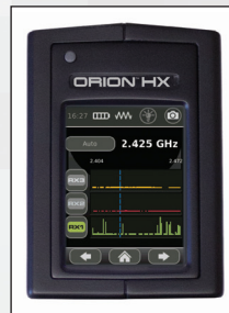
Frequency adjust screen displays Transmit, 2nd, and 3rd frequency ranges.
