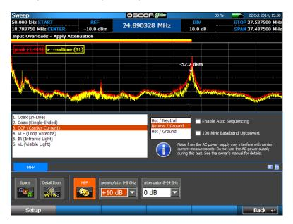
To clear the error, apply just enough attenuation until the input overload warning is no longer displayed. If the signals are still present after the attenuation is applied, they should be considered actual threats.
