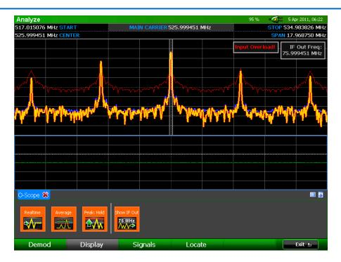
In the screenshot above, a very strong signal has caused an overload condition, creating several false spurs and causing the "Input Overload!" indicator to appear on the spectrum.
