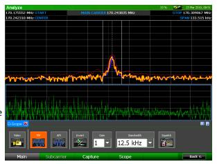
Adjust the threshold to be able to see subtle variations in the RSSI level better. Select the *Threshold* icon. Using the Rotary Knob, adjust the threshold level slightly below the signal level for your transmitter. When finished press the **OK** button.
