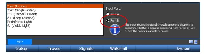
8. Repeat step 5 to save a Peak Trace from Port B. The two saved peaks can now be compared to identify possible suspect signals. A math trace can also be performed on these two peaks (see page 42)
