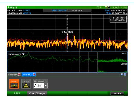
An increased level in the center of the graph is an indication that the demodulated signal correlates with room audio and could be a potential threat. The OSCOR unit will automatically assess the correlation graph and make a determination regarding whether or not the demodulated audio correlates with the ambient room noise. The unit's determination is displayed on the top left hand side of the correlation graph.
