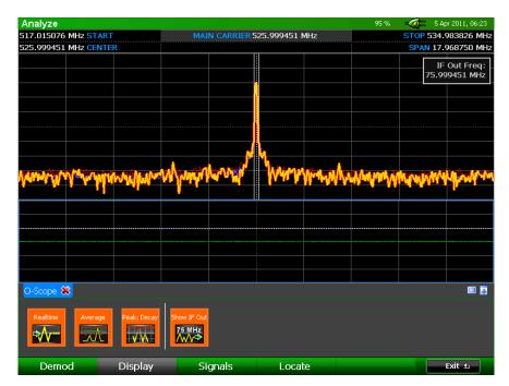
Applying just 10dB of input attenuation has eliminated the overload condition. The overload indicator has disappeared along with all of the false spurs.
