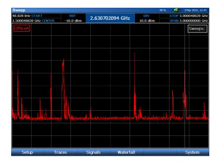
With the peak trace it is also easy to see the frequency hopper at approximately 778 MHz and the burst transmitter at 2.6 GHz, however, we cannot determine any information such as when the transmissions started, how long the transmission continued, nor can we tell that these were frequency hopping and burst signals. We just know that a peak occurred at these frequencies. With the Spectrogram we are able to capture many more details to help with investigating these suspect signals.
