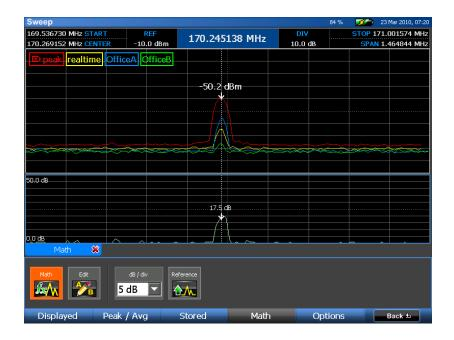
We will now locate this transmitter in Office B using the RSSI Locate function.
