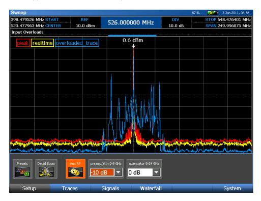
Overload information is stored when peak traces are saved. The screen shot above shows a blue bar above the spectrum to indicate that the stored trace (which is displayed in blue) has an overload condition.
