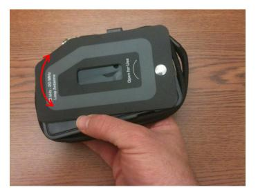
2. On the OSCOR unit, make sure that the "VLF (Loop Antenna)" input is selected.
