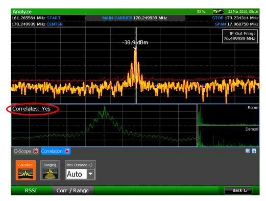
To the right of the correlation graph, the OSCOR unit displays frequency domain graphs of the two audio signals it is comparing to make its correlation determination. The graph labeled "Room" is the room
