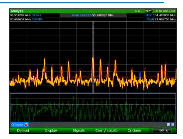
When you first enter Analyze Mode, the spectral graph will appear in the top portion of the screen, just like Sweep Mode. An oscilloscope view of the demodulated signal will appear in the bottom portion of the screen. Also, by default three traces are displayed in the spectral graph in Analyze Mode: the real time trace, the peak trace, and an average trace.
