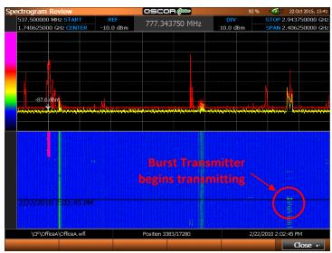
As you move the Spectrogram cursor through the data, pay attention to the displayed traces on the top half of the screen. The red trace is a peak trace of the complete Spectrogram collection session. The yellow trace displays the signals that were present at the time of the timestamp on the Spectrogram cursor.
