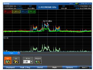
You can use the previous location method of monitoring the signal RSSI level as you walk around the room, but for this example we will use the Live Waterfall Raster to locate the wireless camera.
