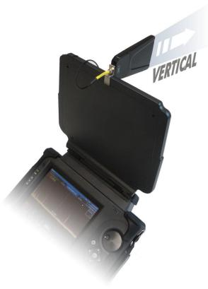
Directional Antenna \* –Clip the included Vivaldi directional antenna to the antenna panel and connect to the 0 – 8 GHz Auxiliary input on the back of the OSCOR unit for improved directivity in the 1.5 GHz to 8 GHz range.
