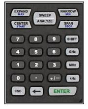
Type in a known FM radio station from the numeric keypad. (95.5 MHz is shown in this example; You should use a known station in your area.)
