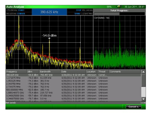
During this 2<sup>nd</sup> part of the process, a correlation graph will be displayed at the top right corner of the screen. If a signal does correlate with room audio, then the text "Correlates" is added to the Threat field for that signal in the signal list.
