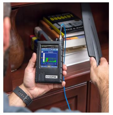
fashion. The ANDRE needed an effective, general-purpose antenna that offered users a reliable, broad frequency range. While the directional antenna included with the ANDRE provides greater detection distance, the Whip outperforms the directional at lower frequencies.
