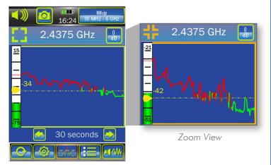
The signal strength histogram displays RF levels over user-selected time intervals ranging from 5 seconds to 24 hours. The adjustable trigger level provides audio, haptic, and visual alerts when RF levels exceed the threshold.
