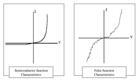
This level of regularity in the junction results in differences in the harmonic signals. When the ORION 2.4 radiates a signal that is returned by the junction in electronics, it results in a strong  $2^{nd}$  harmonic signal and a weak  $3^{rd}$  harmonic. A false junction returns a very weak  $2^{nd}$  harmonic and a strong  $3^{rd}$ .
