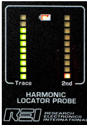
Figure 11: Low Battery Condition
