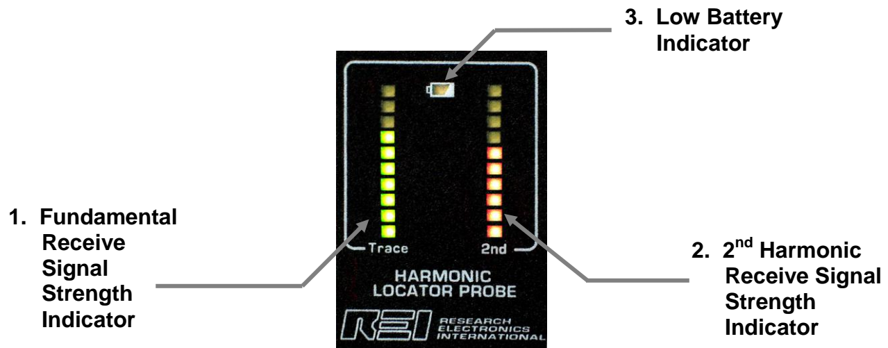
Figure 1: Front Panel Indicators
