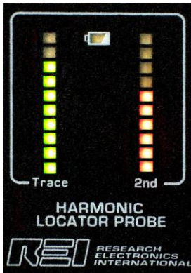
Figure 3: Combination MODE locating a Semiconductor
