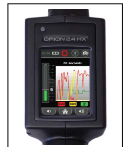
The time graph displays continuous history of harmonic response and power adjustment from 10 - 60 second duration.
