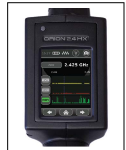
The frequency adjust screen displays Transmit, 2 nd or 3 rd frequency ranges.
