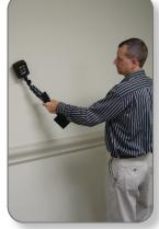
Telescoping antenna pole retracted.
